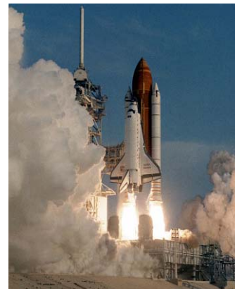
b) Space Shuttle (100 t liquid hydrogen, 600 t liquid oxygen)
