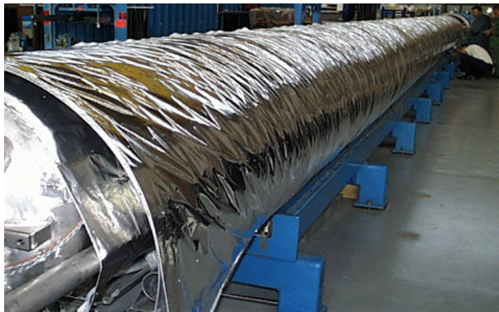
Figure 10 Prefabricated MLI blankets being installed around an accelerator superconducting magnet
